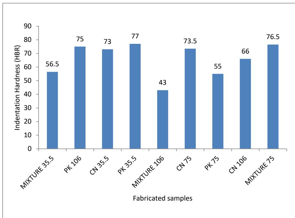
**Figure 3:** Indentation hardness of the fabricated samples
