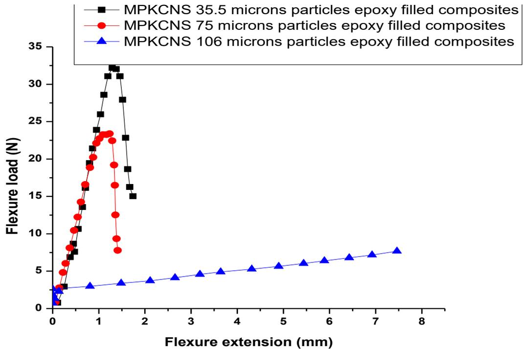
**Figure 6:** Flexure load (N) against flexure extension (mm) of MPKCNS epoxy filled composite
