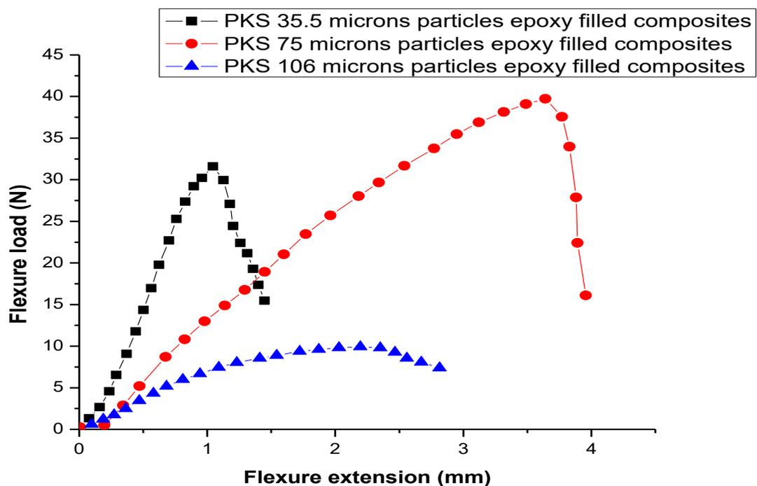
**Figure 4:** Flexure load (N) against flexure extension (mm) of PKS particles epoxy filled composite
