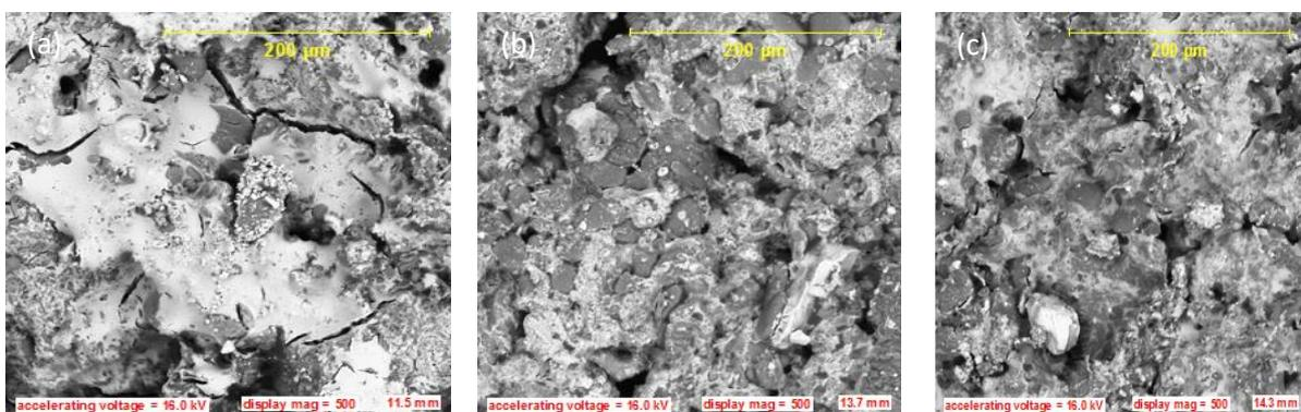
**Figure 9:** SEM image view of fabricated MPKCNS particles epoxy filled composites: (a) 35.5 µm (b) 75 µm and (c) 106 µm
