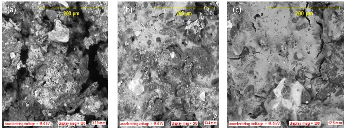
**Figure 7:** SEM image view of fabricated PKS particles epoxy filled composites: (a) 35.5 µm (b) 75 µm and (c) 106 µm
