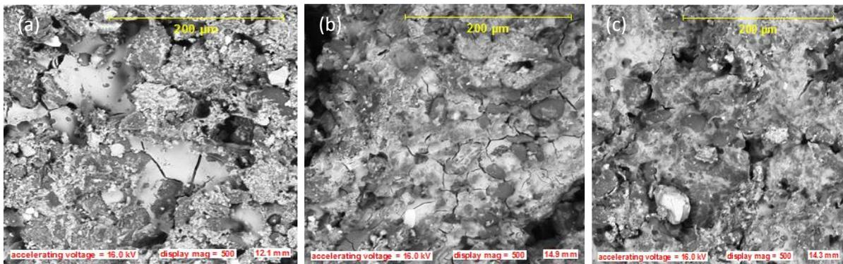
**Figure 8:** SEM image view of fabricated CNS particles epoxy filled composites: (a) 35.5 µm (b) 75 µm and (c) 106 µm
