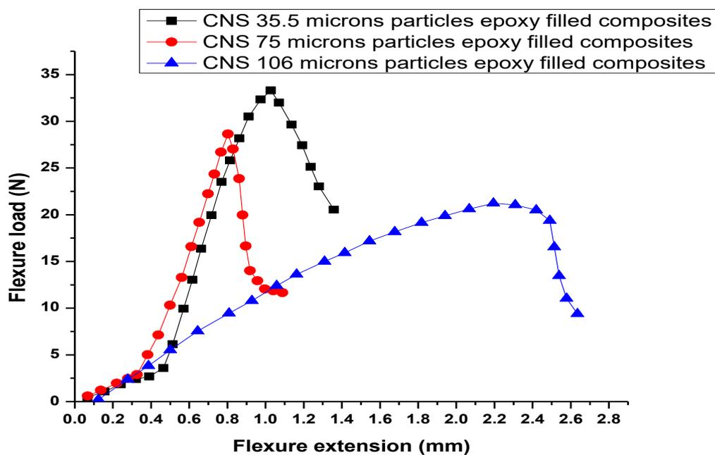
**Figure 5:** Flexure load (N) against flexure extension (mm) of CNS epoxy filled composite
